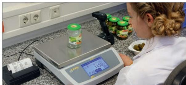
Sample testing of a pre-packaged item with fluctuating packaging weight, such as glass containers, e.g. the tare weight is entered individually for each sample.
