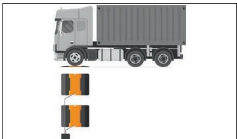
**Asynchronous weighing of individual axles**
