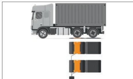
**Asynchronous weighing of double axles which are installed next to each other, using compensation pads**
