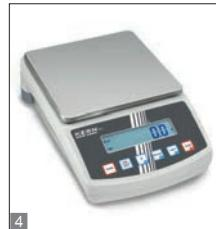
Process reliability thanks to automatic internal adjustment and EC type approval [M]
